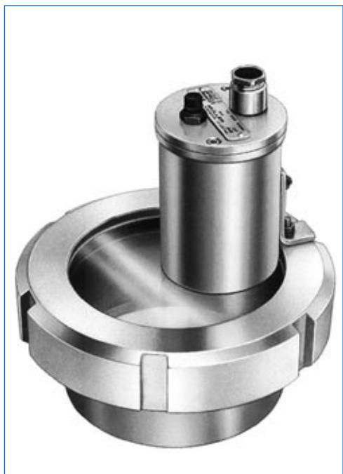
Sightglass light fitting type KVLR 50 HDW1, 50 W, 24 V, with built-in momentary push-button "D", mounted by bracket "W1" on screwed sightglass similar to DIN 11851, DN 100, PN 6, for application "view and light through one assembly".
