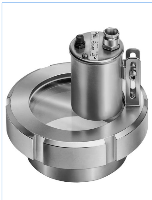
Sightglass light fitting type BKVLR LED DSch1, 24 V, with built-in momentary push-button "D", mounted with tilting hinge "Sch1" on screwed sightglass similar to DIN 11581, DN 100, PN 6, for application "view and light through one assembly".
