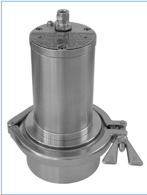
Sightglass light fitting, type EdelEx STERI-LINE 20 dH, 24 V, 20 W, Ex d IIC T4, Ex tD A21 IP65 T130°C, Ex II 2 G + D, on metal fused sightglass, DN 100
