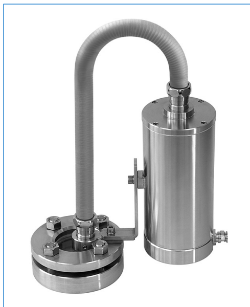
Stainless steel fibre-optic lightpipe light fitting, type fibroLUX® E 5035 W W2 sp, Ex d IIC T4, Ex tD A21 IP65 T130°C, Ex II 2 G + D, 35 W, 12 V DC, fixation of the light source by bracket "W", fixation of the lightpipe by universal support "W2" onto sightglass to DIN 28120, DN 40, PN 10
