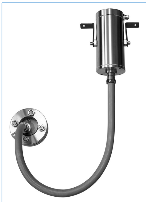
Stainless steel fibre-optic lightpipe light fitting for use in hazardous areas, type fibroLUX® E 5035 X1 W2, Ex d IIC T4, Ex tD A21 IP65 T130°C, Ex II 2 G + D, 35 W, 230 V, fixation of the light source by fixation legs "X1", fixation of the lightpipe by universal support "W2" onto sightglass to DIN 28120, DN 40, PN 10
