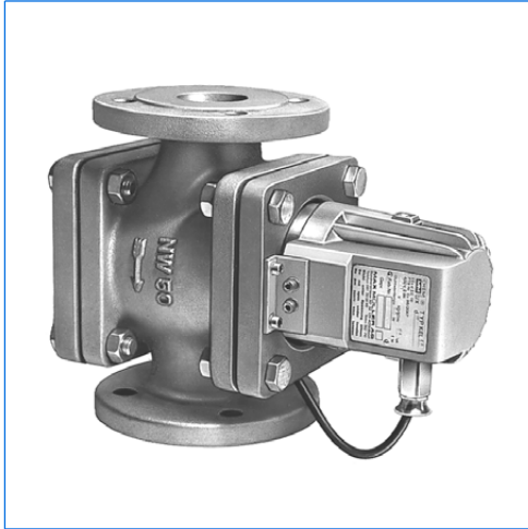
Sight flow indicator, type FDE 50, with sightglass light fitting type FKEL 5 dH WM, Ex d IIC T6, Ex tD A21 IP65 T80°C, Ex II 2 G + D, 230 V, 5 W, with opal glass screen «M»
