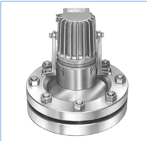
VETROLUX® illuminated sightglass unit, consisting of sightglass to DIN 28120, DN 150, PN 10, with mounted CHEMLUX® light fitting, type KEL 20 deH Sch B, 230 V, 20 W, Ex de IIC T4, Ex tD A21 IP65 T130°C, Ex II 2 G + D, with anti-dazzle shield "B", in version "view and light through one assembly"
