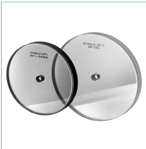
Sightglass discs similar to DIN 8902 or DIN 7080 with central bore hole \varnothing 10,5 mm to fit our wipers of the series W / WD.
