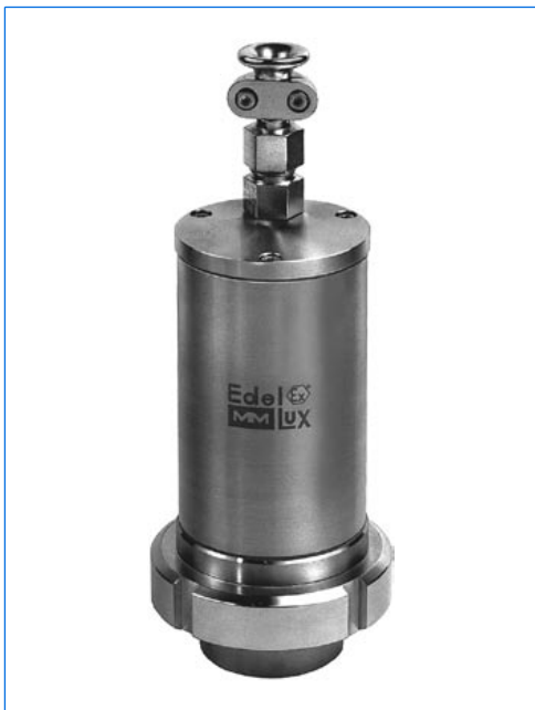
Sightglass light fitting type EdelEx 10 dH R50 K1, 10 W, 230 V, Ex d IIC T4, Ex tD A21 IP65 T130°C, Ex II 2 G + D, with intermediate flange collar fixation "R", mounted onto a screwed sightglass similar to DIN 11851, PN 6, DN 50.
