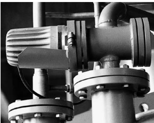
CHEMLUX ® sightglass light fitting, type L 20 deH M sp, 20 W, 24 V, Ex de IIC T5, Ex tD A21 IP65 T95°C, Ex II 2 G + D, mounted with an opal glass screen "M" on a pipeline flow indicator
