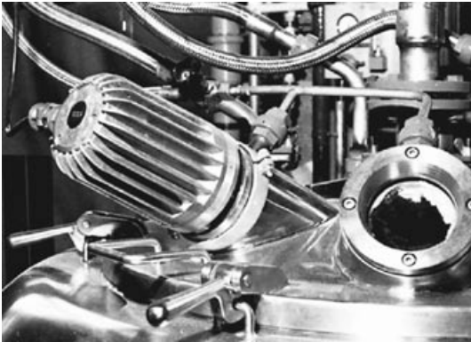
CHEMLUX ® sightglass light fitting, type L 20 dH Sch, 20 W, 230 V, Ex de IIC T5, Ex tD A21 IP65 T95°C, Ex II 2 G + D, with fixation "Sch" on a basket centrifuge
