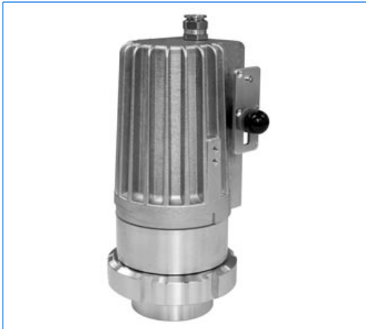
Type FHEL 35 dhVRK1, Ex d IIC T4, Ex tD A21 IP65 T130°C, Ex II 2 G + D, 230 V, 35 W, halogen version, with timer "V", on screwed sightglass similar to DIN 11851, DN 65, PN 6. Fixation with intermediate flange collar "R".
