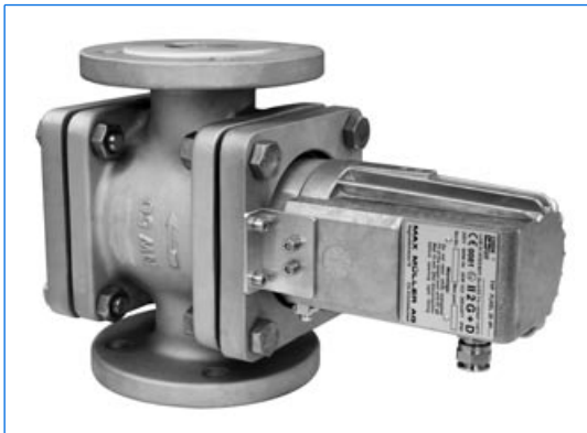
Type FHEL d LED-F MWSp, Ex d IIC T6, Ex tD A21 IP65 T80°C, Ex II 2 G + D, 230 V, ca. 2 W, LED version, with optical glass "M", on pipeline flow indicator type FDE 50, DN 50.
