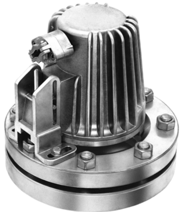
Type F 20 dHSchU, Ex d IIC T5, Ex tD A21 IP65 T95°C, Ex II 2 G + D, halogen bulb, 230 V, 20 W, with built-in timer «U», mounted on sightglass to DIN 28120, DN 125, PN 10, with tilting hinge fixation "Sch"
